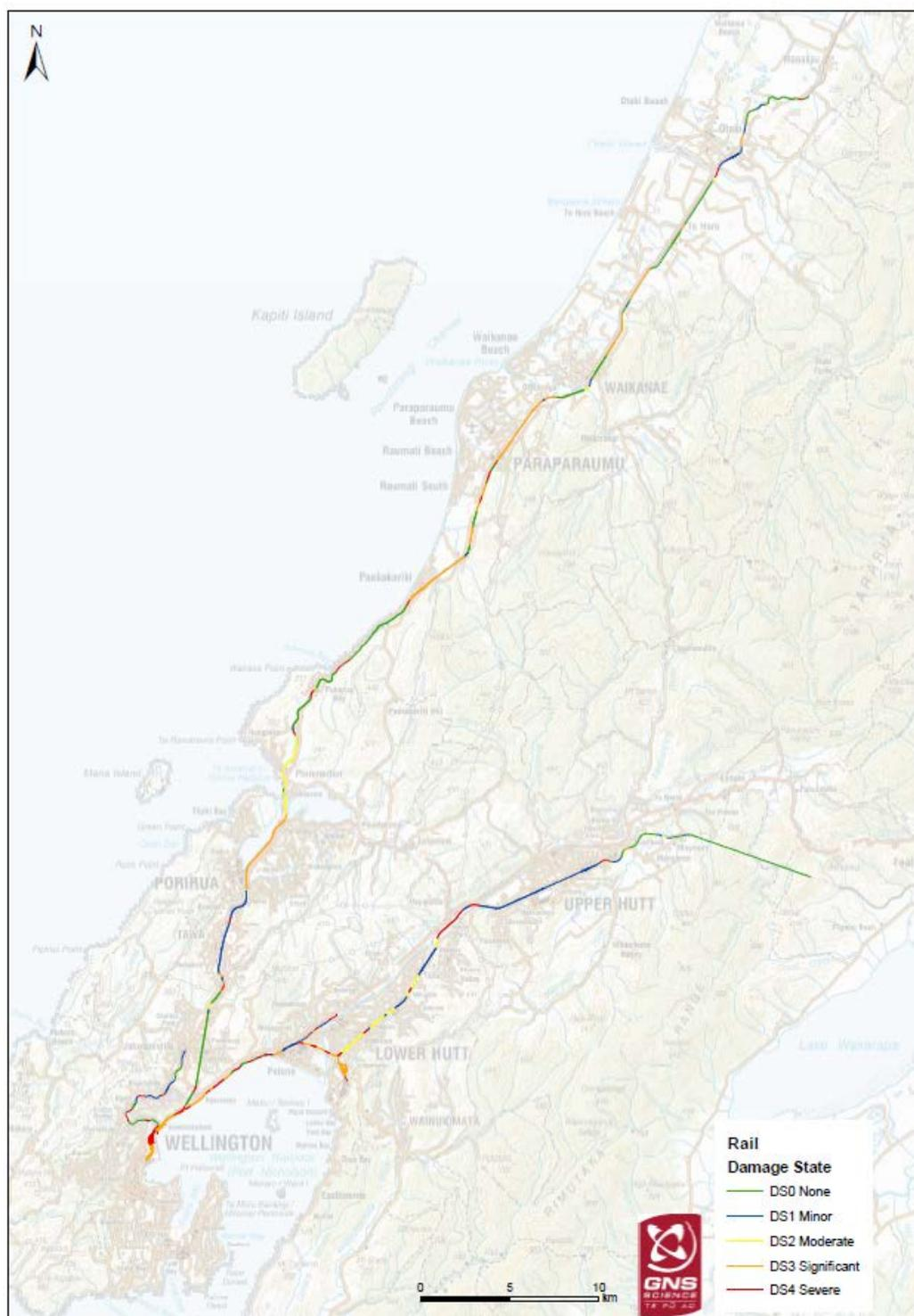
**Figure 5.4** Modelled damage to the Wellington Region rail network.
