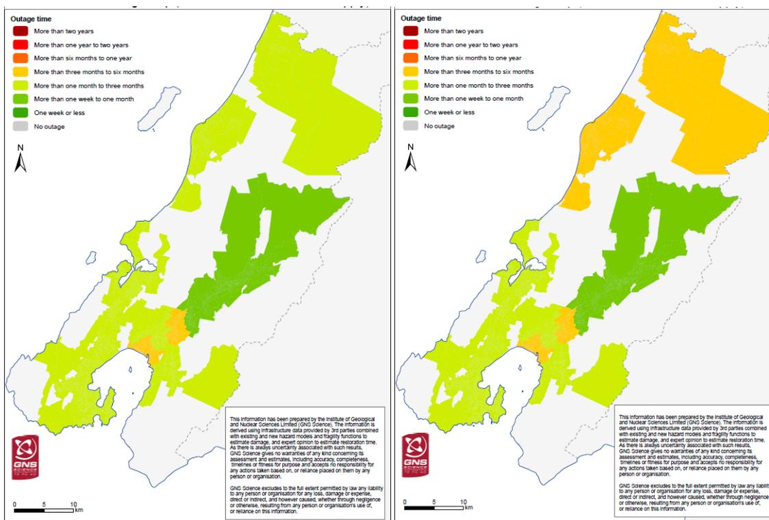
Figure 6.17 Outage map for non-potable (left) and potable (right) water services for the preferred programme.
