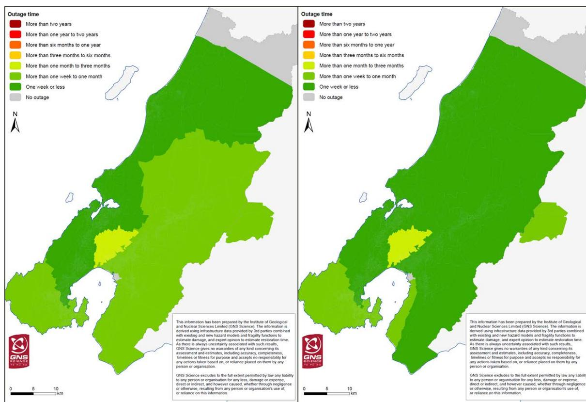
**Figure 6.3** outage times for fuel service to critical and general customers with low investment interventions (left) and high investment interventions (right).
