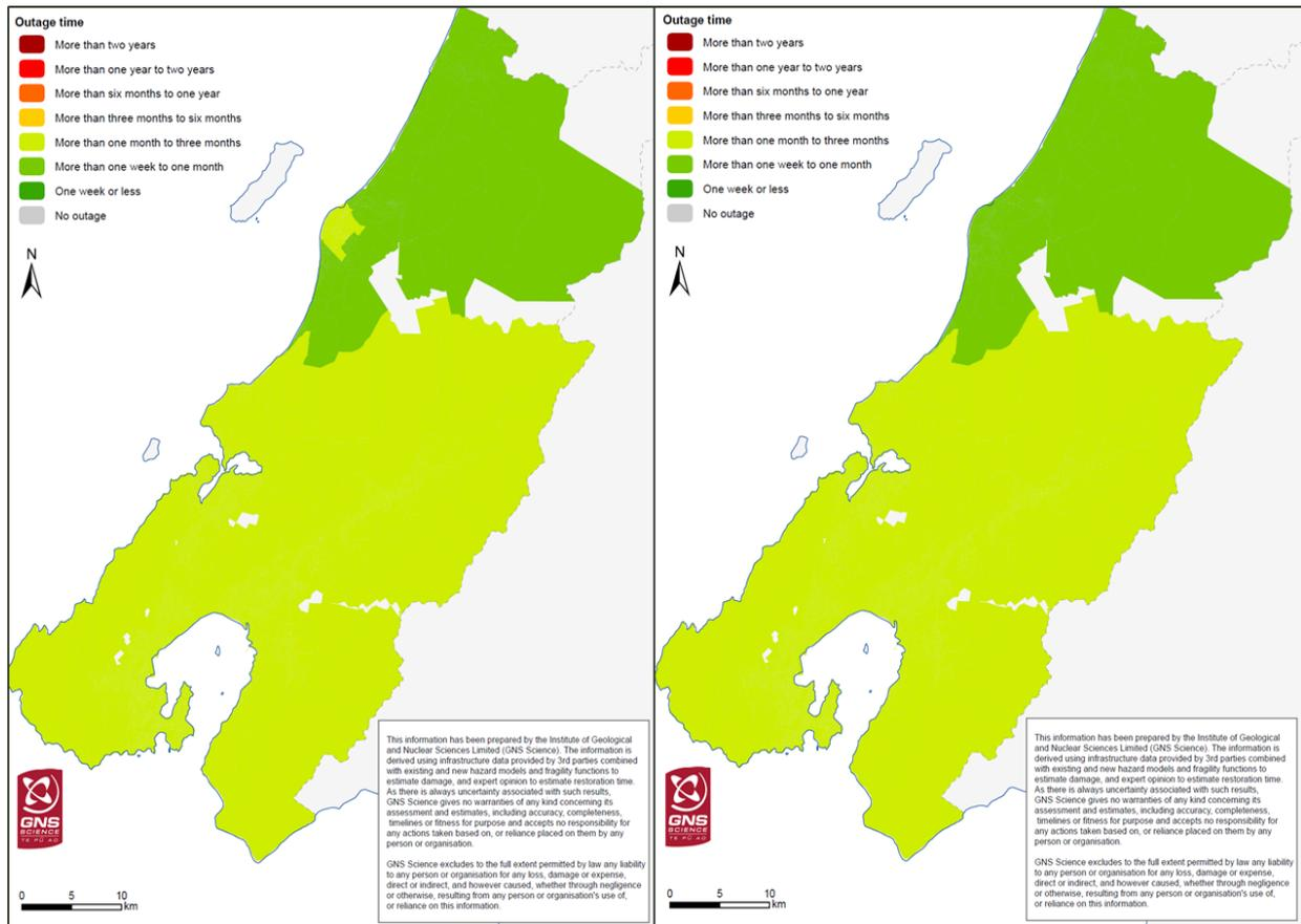
**Figure 6.7** Updated electricity network outage for low (left) and high (right) investment programmes.
