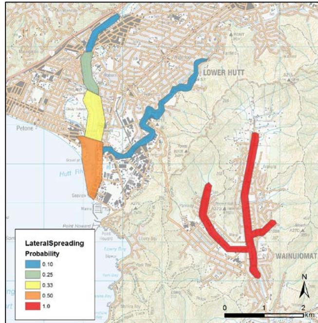
**Figure 4.4** Map showing lateral spreading zones of varying occurrence probabilities in Lower Hutt and Wainuiomata.
