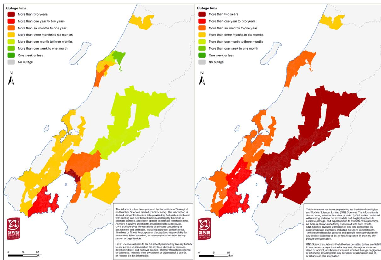
Figure 6.19 Outage times for waste water collection (left) and treatment (right) services.
