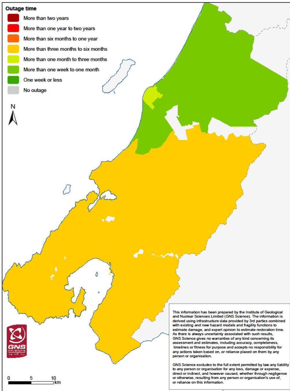
Figure 6.6 Outage map for electricity service for base-case scenario.
