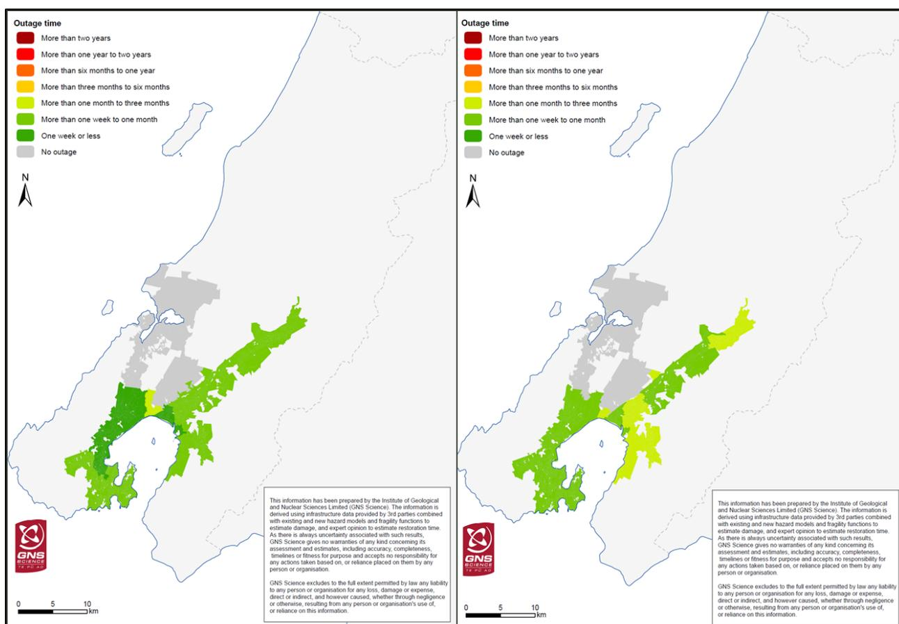
**Figure 6.24** Outage times for gas to critical (left) and general (right) customers incorporating the intervention project to supply critical customers with bottled gas or isotainers.
