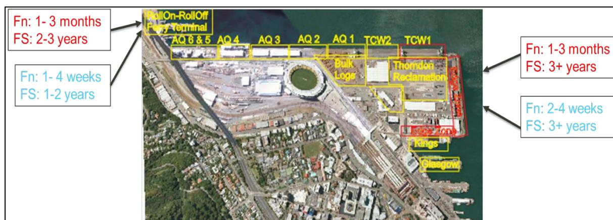
**Figure 5.5** Restoration times for port assets in Wellington. Red text is base-case outage times, blue text is intervention and preferred programme outages.
