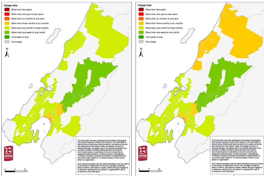
**Figure 6.16** Outage map for non-potable (left) and potable (right) water services for low and high investment intervention programmes.
