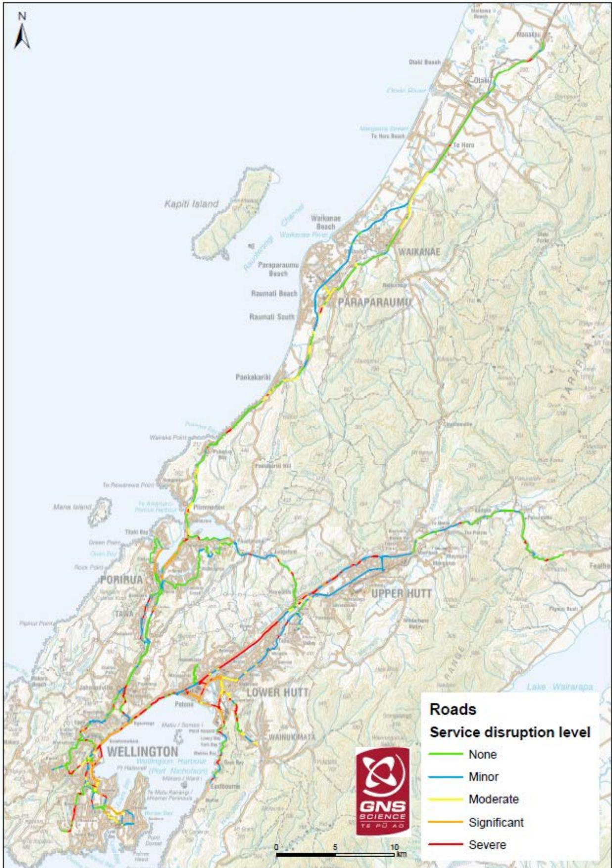
Figure 5.2 Service Disruption Level for modelled roads.
