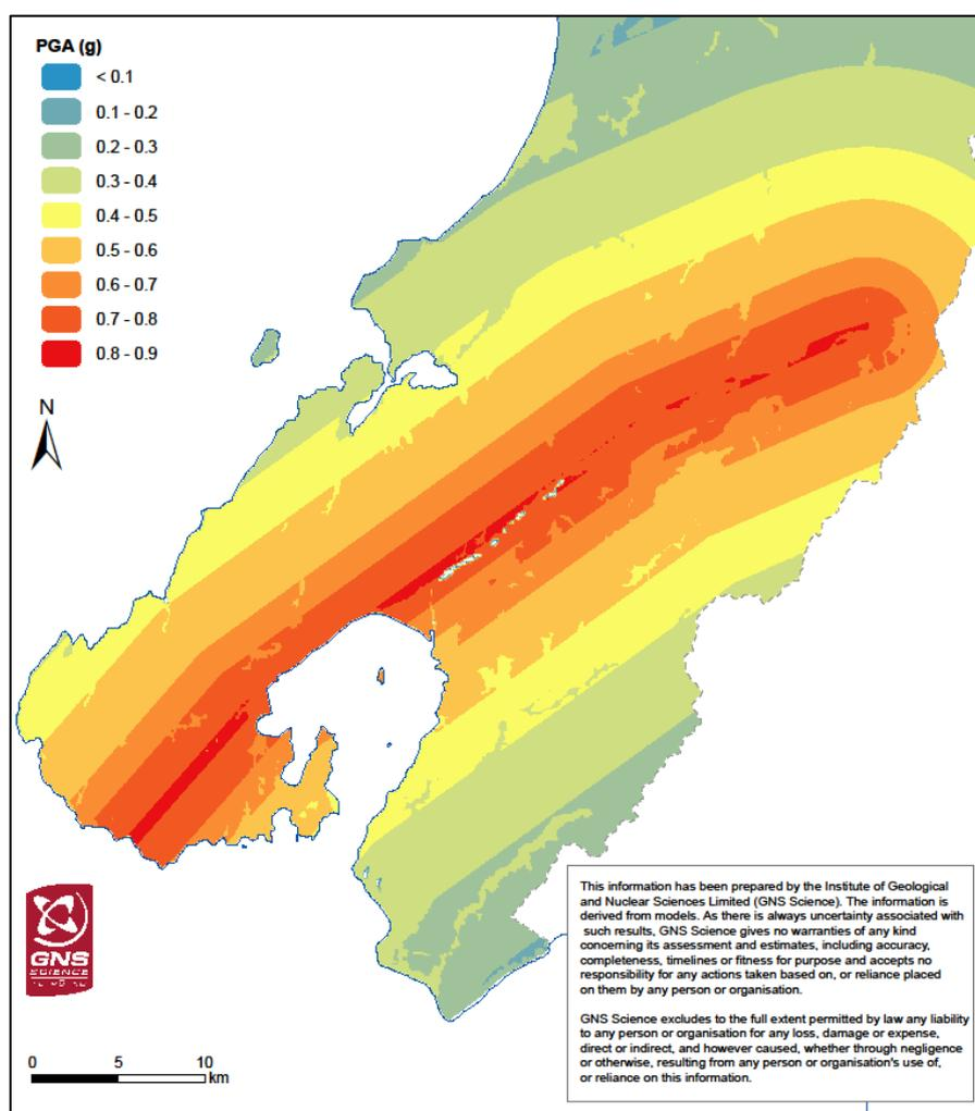
**Figure 4.2** Peak Ground Acceleration (PGA) for Wellington Fault Scenario.
