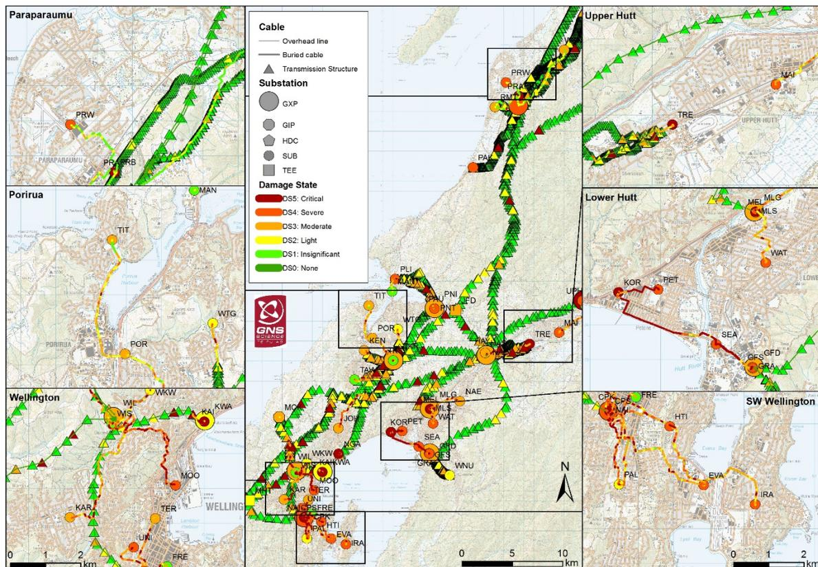
**Figure 6.4** Modelled damage to the Wellington Region electricity network in the base case.
