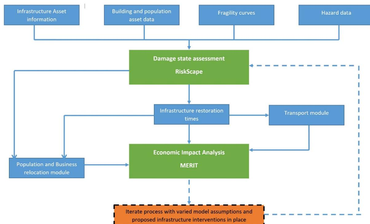
**Figure 1.1** Linkages between the various stages of damage loss assessment and economic impact analysis for the Wellington Resilience PBC.
