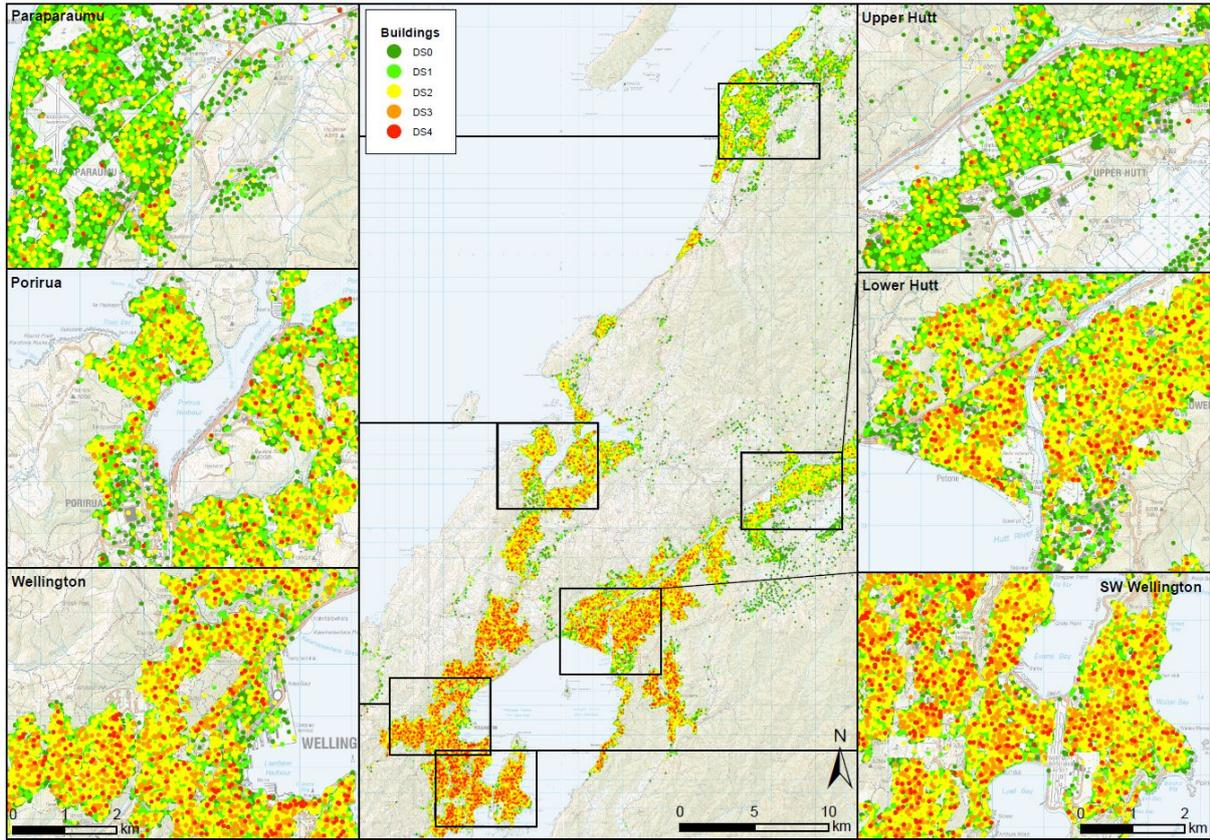
Figure 7.1 Modelled damage states for Wellington Region buildings.
