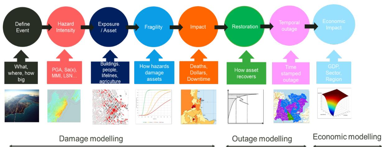
**Figure 2.2** Workflow of modelling for temporal outage of lifelines.
