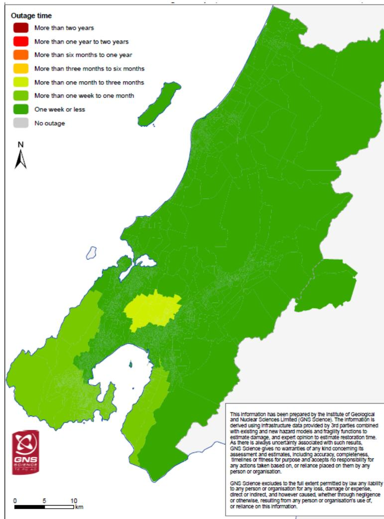
**Figure 6.12** Outage times for telecommunication services (data, cellular and landline) for preferred programme.
